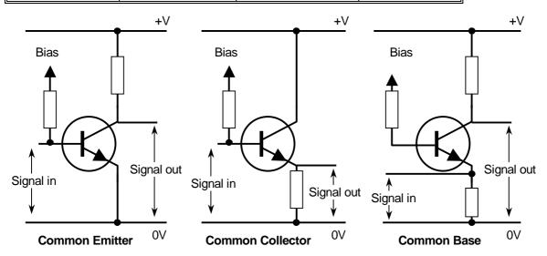
**The Three Modes Of Connection For Transistor Amplifiers**
